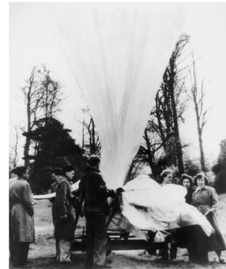
Figure 1 A balloon ready for the ascent in the Sardinia area in July 1953. For the first time, emulsion stacks were made up of 40 stripped emulsions bound together between thick glass plates, wrapped and sealed and subsequently marked with X-rays.
