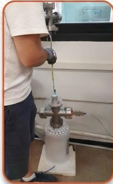
Sensor Insertion into Pressure Vessel.
