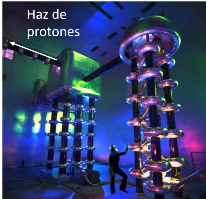
750 kV Cockcroft-Walton generator at Fermilab (Proton source)
