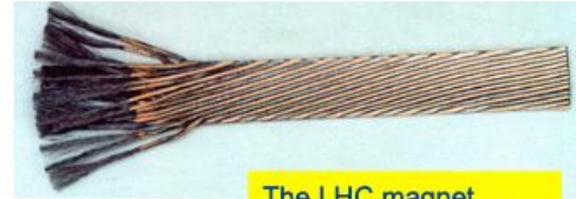
The LHC magnet superconducting cable
