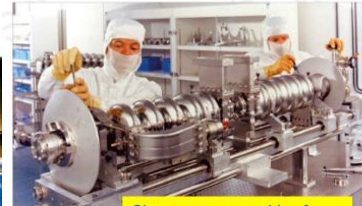
Clean room assembly of superconducting RF cavities
