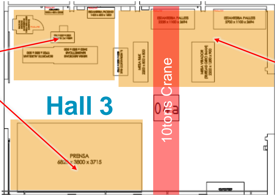
3700 tons with 10 cylinders (5 pairs) Mould up to 2500x1000x400 mm (LxWxH) & 2 tons
