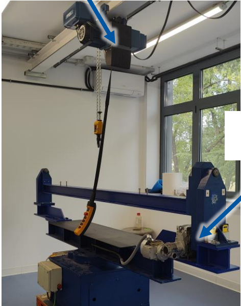
Winding machines and pay-off machines for pulling cable tension (closed-loop control)
