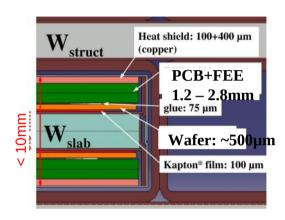
Semi-conductor readout Typical segmentation: 0.5x0.5 cm<sup>2</sup>
