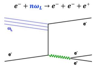
Positron-electron pair production not accessible in "standard" QED... ⇒ "smoking gun" for non-linear processes...
