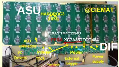
New Detector InterFace (DIF) board able to manage the 30000 channels of a single RPC 3x1m<sup>2</sup>
