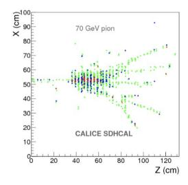
48-layer HCAL prototype, ~440000 readout channels (SemiDigital)
