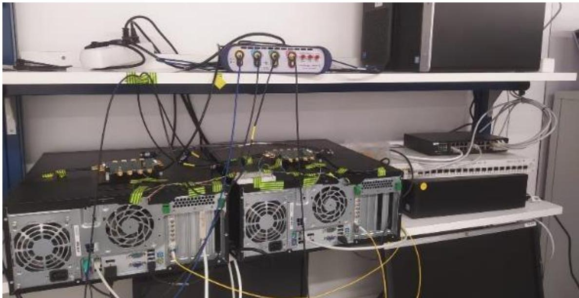
Phase A: Coaxial clock distribution with external clock synthesizer (40 MHz) using the Si5338 as 1:N fanout (transparent)
