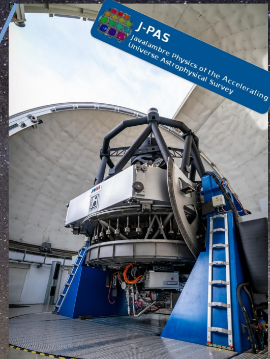
JST250 Ritchey-Chrétien plus Field Corrector Diameter = 2,55 m FoV = 3 deg \varnothing F/3,5 M2 hexapod
