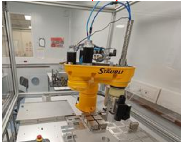
Glue deposition via stamp Micrometric precision using robot
