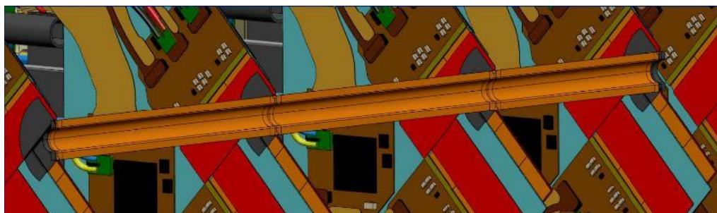
Conceptual design for a lightweight cylindrical RF-shield between the LHC beamline and the Upgrade II VELO modules
