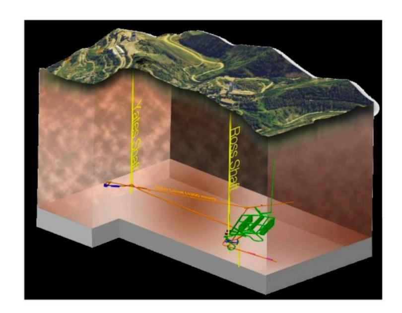
~70kt of LAr deployed in 4 modules in two massive caverns 1.5km underground and 1300km away from FNAL;
