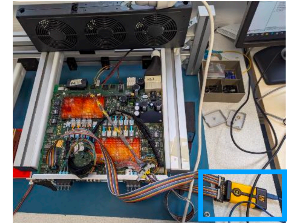
XJTAG setup with the LASP T2
