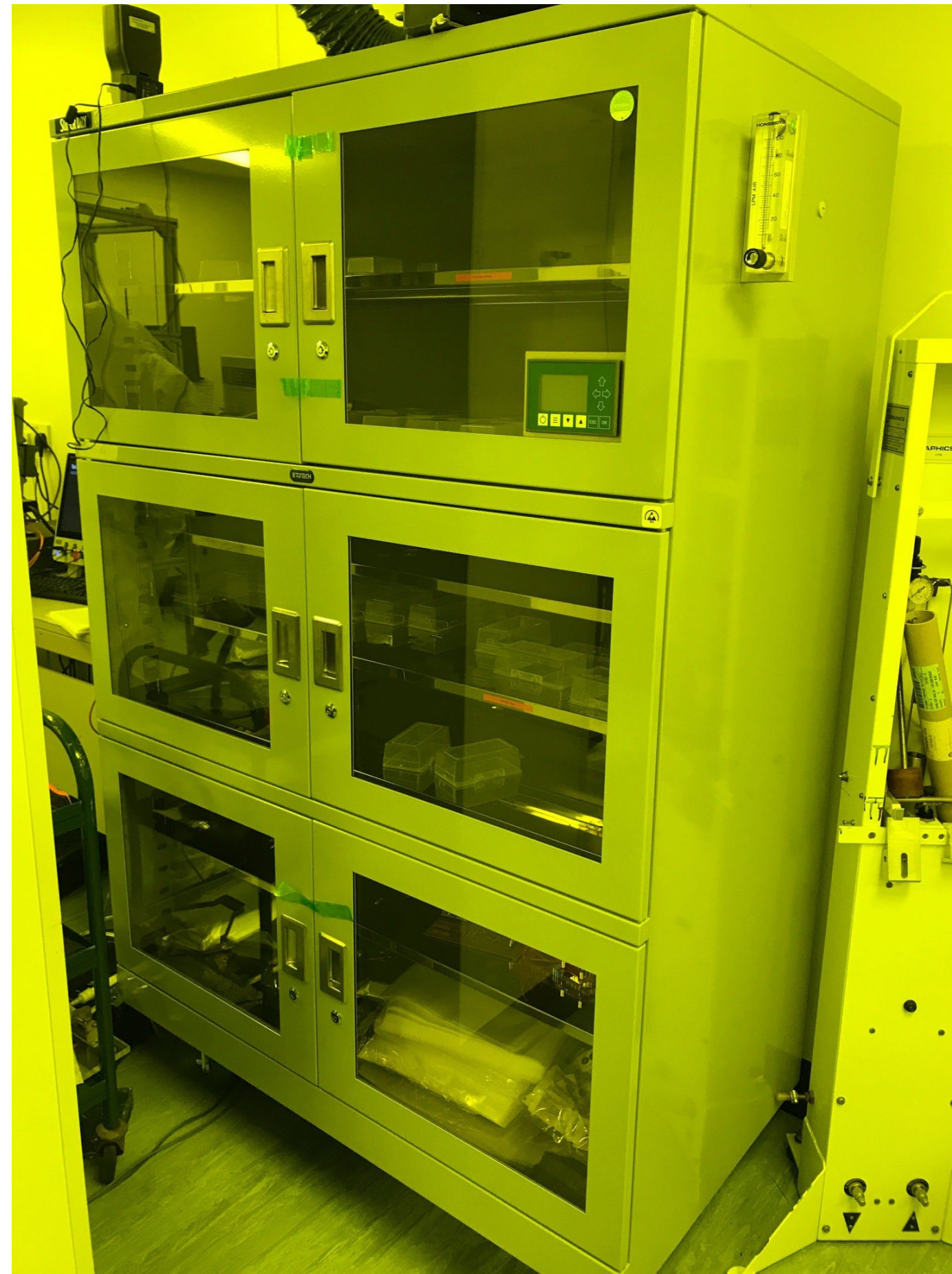
PDU storage in nitrogen-purged conditions
