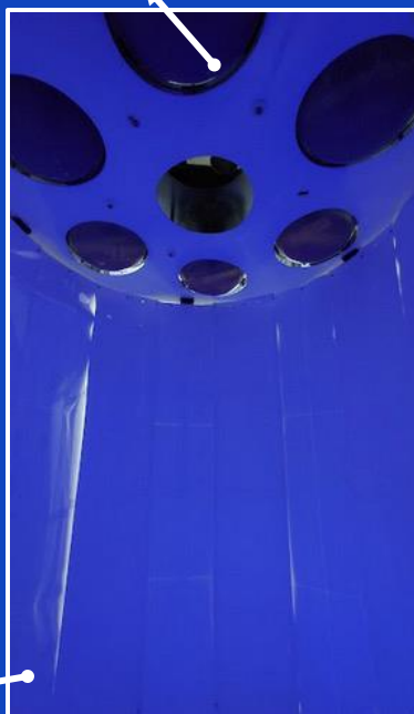
PMT Plane with reflector coated with TPB
