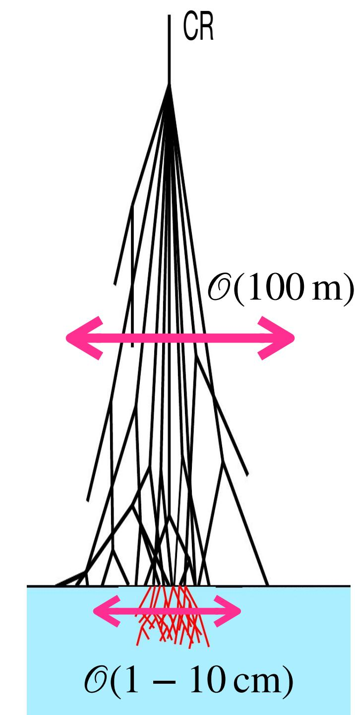
**In-ice emission should be more coherent than the in-air component**
