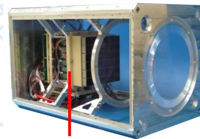
2304-pixel focal surface made of 36 MAPMT modules (6 x 6), each of 64 (8x8) PMT "pixels"
