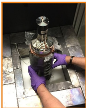
CsI detector (COHERENT collaboration)
