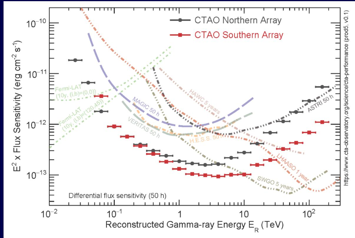
The differential sensitivity is defined as the minimum flux needed by the CTAO to obtain a 5-standard-deviation detection of a point-like source.
