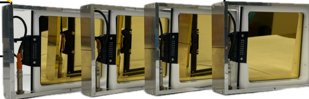
Silicon dE telescope (4 × 600- \mu\text{m} Si)
