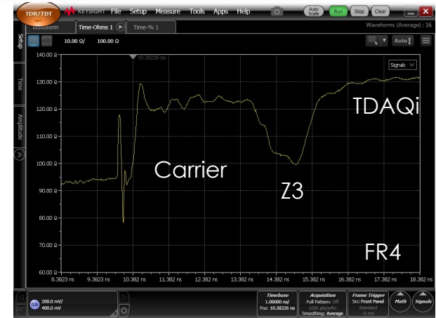
Differential impedance of the longest trace connecting AMC bay 4 and the TDAQi plugged in the Zone 3
