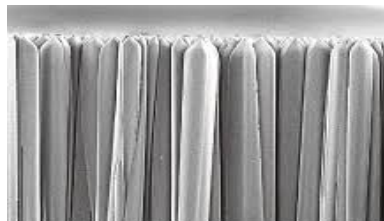
SEM image of CsI crystals
