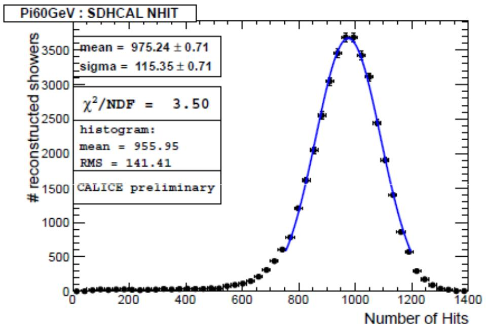
Gaussian Fit in the range of 2 standard deviations around the mean value
