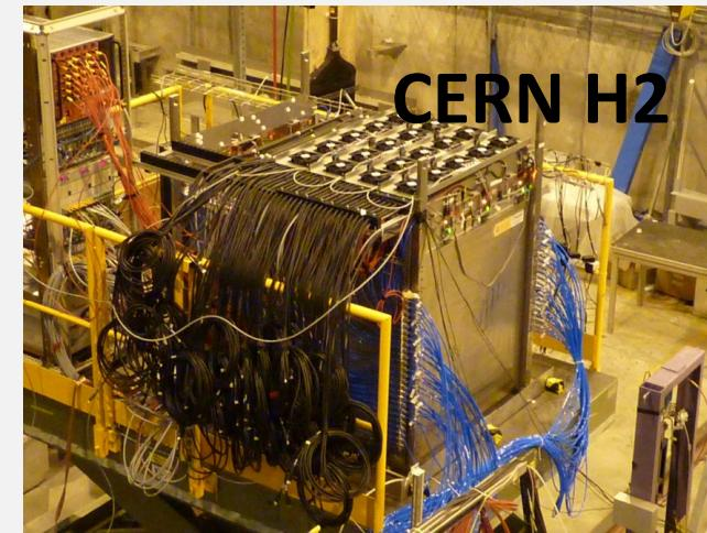
Gaseous detectors like **GRPC** (Glass Resistive Plate Chambers) are homogenous, cost-effective, and allow high longitudinal and transverse segmentation.
