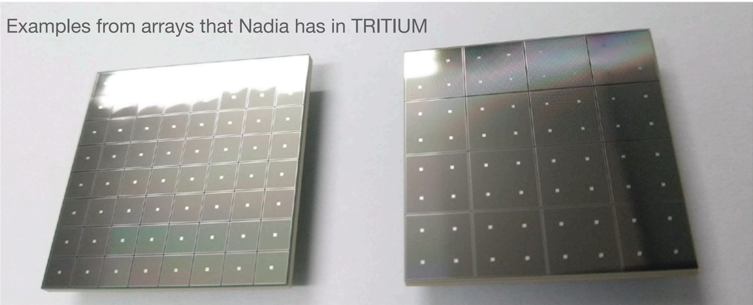
S13361-3075AE-08 MPPC array, 8x8 1156€ + IVA
