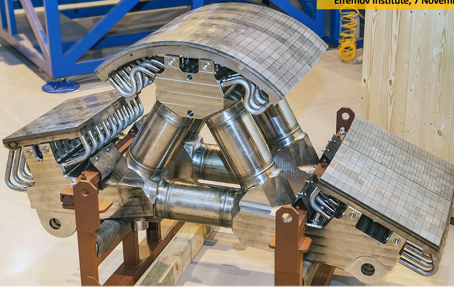
Russia completed Full Scale Prototype of the divertor dome: arrived at ITER on 14 December 2021
