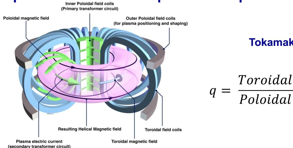
$$q = \frac{\text{Toroidal turns}}{\text{Poloidal turns}} \geq 2$$
