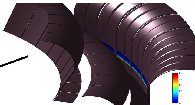
$q_{\text{div}} \sim 50 \text{ MWm}^{-2} \rightarrow$  similar to heat flux on sun's surface ( $60 \text{ MWm}^{-2}$ )
