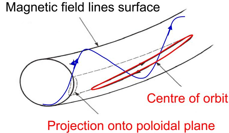
$$\delta r_p = a/R B_t/B_p \quad \rho < 3 \rho \text{ (tokamak)}$$
