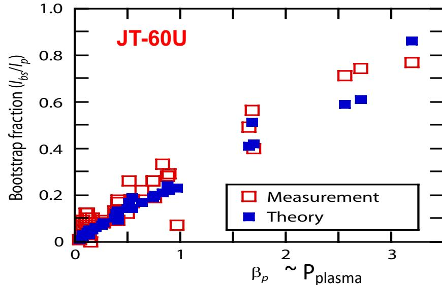
Bootstrap current is a key ingredient to achieve  $Q = 5$  steady-state operation in ITER
