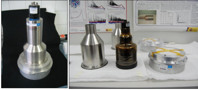
Figure 2. (Left) Picture of the first detector prototype manufactured by St. Gobain. (Right) Detector components ready for assembling.
