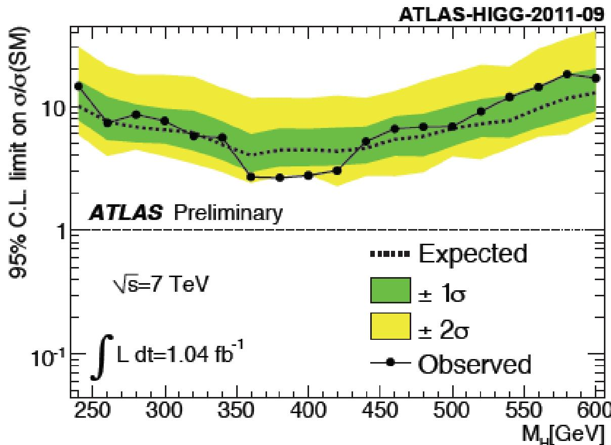
**Sensitivity is 5-10 x SM. Downward fluctuation around 400 GeV**
