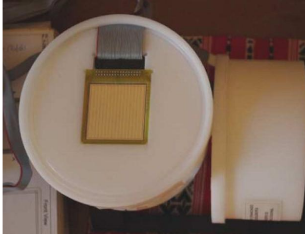
Si strip detector inside a cilindrical phantom
