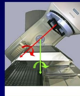
Rotations around the mechanical isocentre
