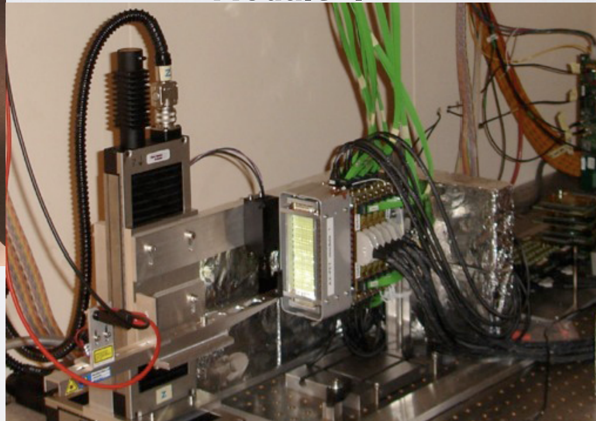
0.9 \times 3 \times 40 \text{ mm}^3 WLS strips from EJEN are readout by 1.19 \times 3 \text{ mm}^2 MPPC (1200 pixels).
