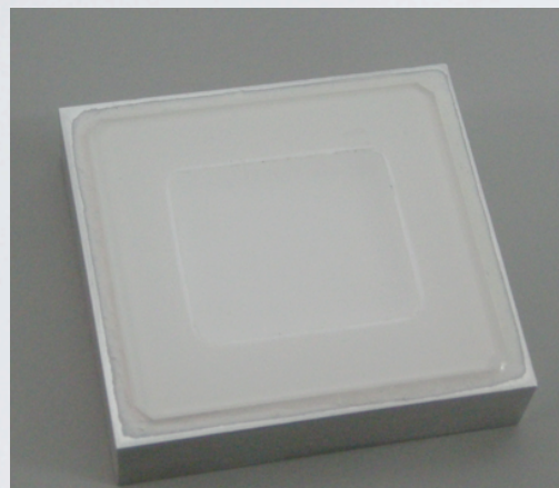
LaBr3 slab 16x18x5 mm 3 encapsulated by reflective material.
