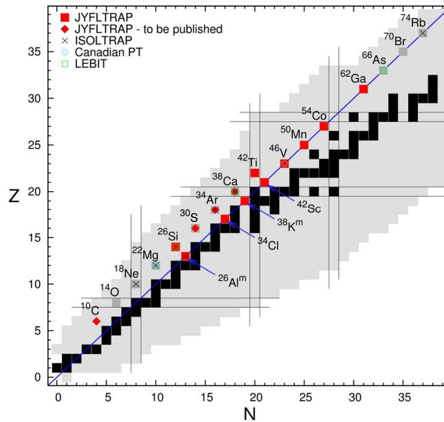
**FIGURE 1.** Chart of the nuclei where superallowed beta emitters have been indicated. The Q values of nuclei marked with red color have been measured with JYFLTRAP, with cross at ISOLTRAP (ISOLDE, CERN), with circle at Canadian PT (Argonne) and with squares at LEBIT (MSU).
