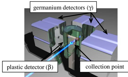
**FIGURE 1.** Schematic view of the experimental setup used in Jyväskylä experiments: the isotopes are deposited on the tape and the collection point is surrounded by the beta detector. Germanium counters are used to measure the gamma de-excitation for branching ratio determinations.
