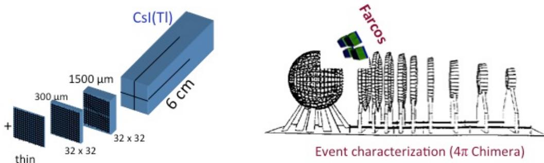
**FIGURE 2.** Left panel: Schematic view of the expected design of Farcos telescopes. Right panel: Coupling of the Farcos array to the Chimera detector at the LNS of Catania.
