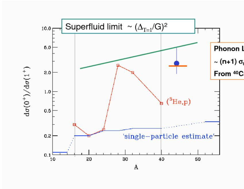
**FIGURE 3.** Systematics of  $\sigma(0^+)/\sigma(1^+)$  for nuclei up to  $^{40}\text{Ca}$ . The preliminary result for the  $^{44}\text{Ti}$  experiment is also shown. Single-particle and superfluid ( $T=1$ ) limits are indicated as references.
