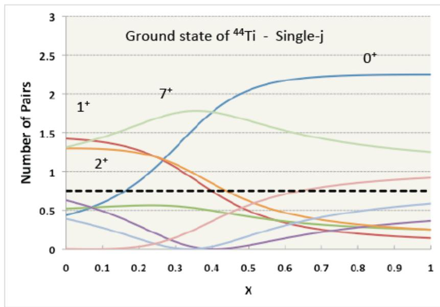
**FIGURE 1.** Number of pairs of a given spin in the ground state of  $^{44}\text{Ti}$  as a function of the relative strength of  $T=0$  vs.  $T=1$  pairing, measured by the parameter  $x$ . Pure isoscalar corresponds to  $x=0$  and pure Isovector  $x=1$ .
