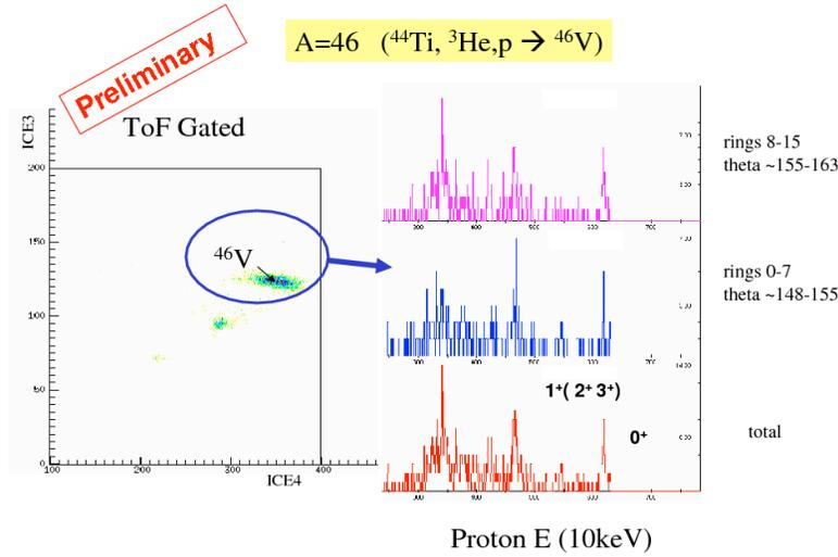
**FIGURE 2.** Proton spectra for the  $^{44}\text{Ti}$  reaction. These are obtained by selecting  $^{46}\text{V}$  recoils as seen by the FMA
