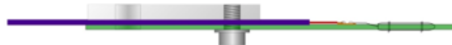
Fig. A2.3. Details of the cable restraining system at the sensor are shown. By sandwiching the cable between the PCB and stainless steel rod mount, the sensor soldering joints are tension free during construction and installation.
