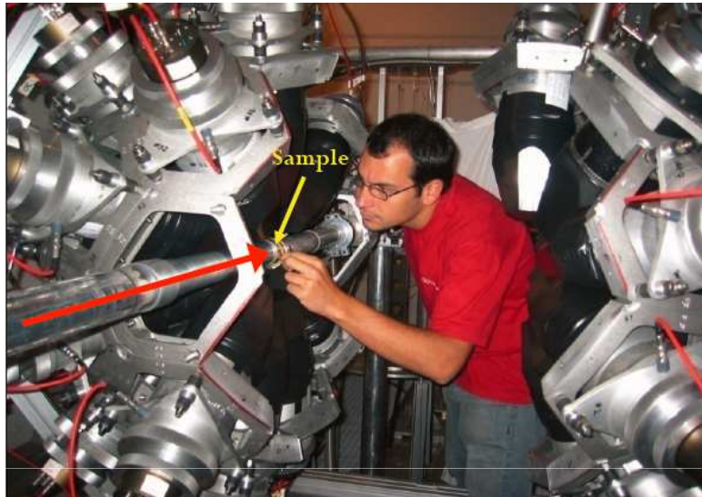
C 6 D 6 based Total Energy Detector (TED)
