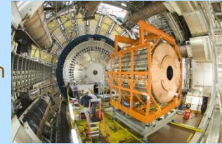
SCT+TRT Endcap installed with in ATLA April-2007
