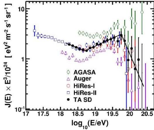
Figure 9: UHECR flux ( $\times E^3$ ) vs  $\log E$  (eV) from five years of TA SD data overlaid with results from HiRes [6], AGASA [5], and Auger [9].
