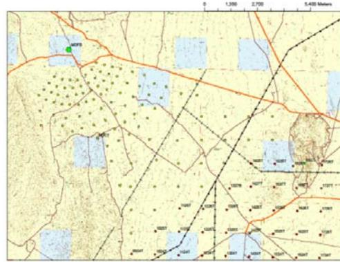
Figure 2: layout of the TALE surface detectors. The Middle Drum (MD) FD site is shown by the square circle in the upper left, and the TALE SD units fan out in a graded pattern to the south of MD. The array shown in the lower right hand of the map are those of the main TA SD array with 1.2km spacing between nearest neighbors.
