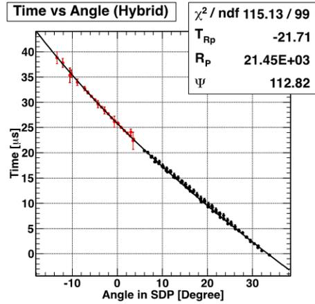
Figure 6: Plot of signal arrival time for FD pixels (black points) vs. the angle measured from the horizon to the pixel, along the shower-detector plane (SDP). This fit is made an order of magnitude more precise by the inclusion of the times of the SD hits (red points).
