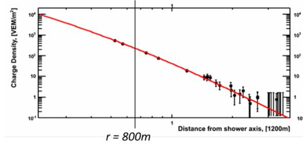
Figure 4: Plot of particle density vs. distance to the shower axis (the lateral density distribution) for the event shown in Figure 3. The density at 800m (S800) is interpolated from the fit, and used with the zenith angle of the shower to obtain the raw shower energy from a look up table.
