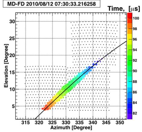
Figure 5: Event display of an FD event from the Middle Drum site. The circles indicate hit PMT pixels. The size of the circles gives the signal strength, while the colors indicate arrival times. The solid curve gives the fitted shower-detector plane.
