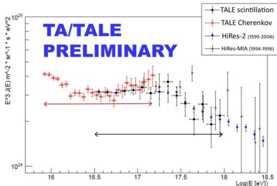
Figure 14: Preliminary monocular energy spectrum using data from the ten new TALE high-elevation telescopes only. The black data points show the spectrum of events analyzed from primarily scintillation (fluorescence) light. The red points show the spectrum from the analysis of Cherenkov-light dominated events. Previous spectra from HiRes-2 and HiRes-MIA are also shown.
