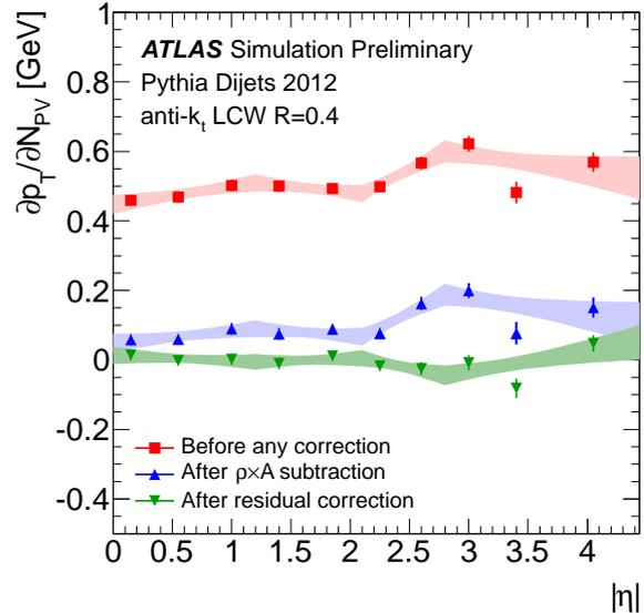
Figure 1: The slope of the jet  $p_T$  dependence on  $N_{PV}$  as a function of jet pseudorapidity before any correction, after jet-area-based correction, and after residual offset correction in simulated dijets events, [8].
