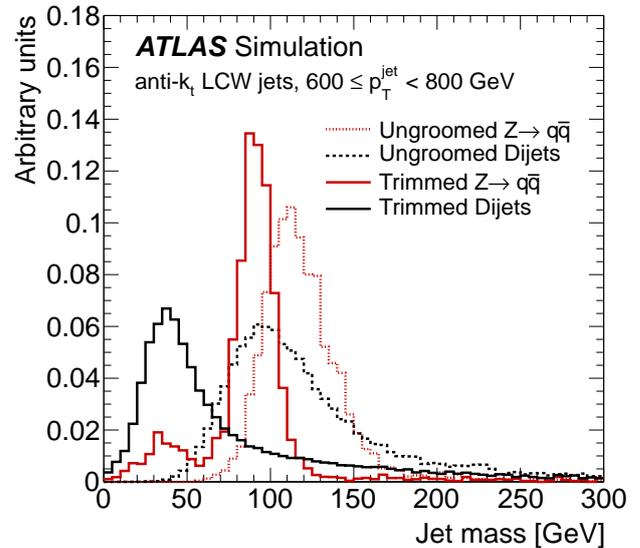
Figure 6: Leading- $p_T$  jet mass distribution for simulated hadronically decaying  $Z$  boson signal events (red) compared to dijet background events. The dotted lines show the ungroomed jet distributions, whereas the solid lines show the trimmed jet distributions, [15].
