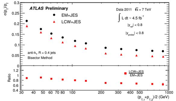
Figure 4: Fractional jet energy resolution for anti- $k_t$   $R = 0.4$  jets as a function of the average jet transverse momenta measured with the bisector in-situ technique using the EM+JES calibration (circles) and the LCW+JES calibration (triangles) with 2011 data. The bottom plot shows the ratio as a function of the average jet transverse momenta, [12].
