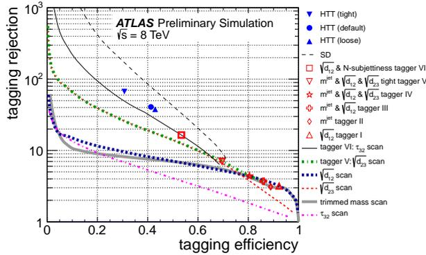
Figure 7: The dependence of the light-jet rejection rate on the top-jet tagging efficiency for different taggers. All substructure taggers and scans use trimmed anti- $k_T$   $R = 1.0$  jets. The HEPTopTagger (points labelled HTT) uses C/A  $R = 1.2$  jets that are geometrically matched to the anti- $k_T$  jets, [21].
