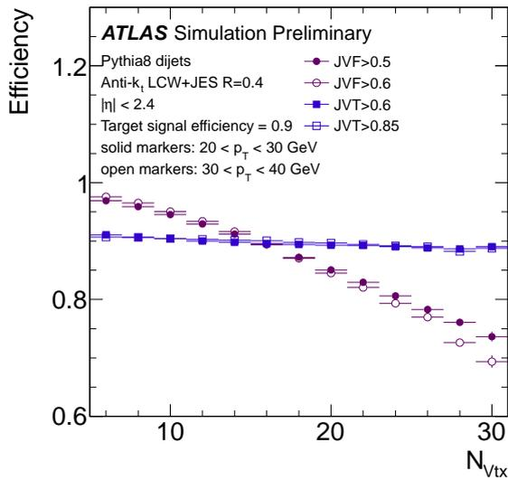
Figure 5:  $N_{PV}$  dependence of the hard-scatter jet efficiency for fixed cuts of JVT (blue) and JVF (violet) chosen such that the inclusive efficiency is 90%. The cut values imposed on JVT and JVF, which depend on the  $p_T$  bin, are specified in the legend, [13].
