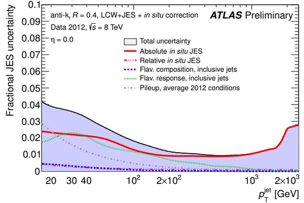
Figure 3: Fractional jet energy scale systematic uncertainty components as a function of  $p_T$  for anti- $k_t$  jets with radius parameter of  $R = 0.4$  at  $|\eta| = 0$  calibrated using the LCW+JES calibration scheme. The total uncertainty (all components summed in quadrature) is shown as a filled blue region topped by a solid black line. Average 2012 pileup conditions were used, and topology dependent components were taken from inclusive dijet samples, [10].
