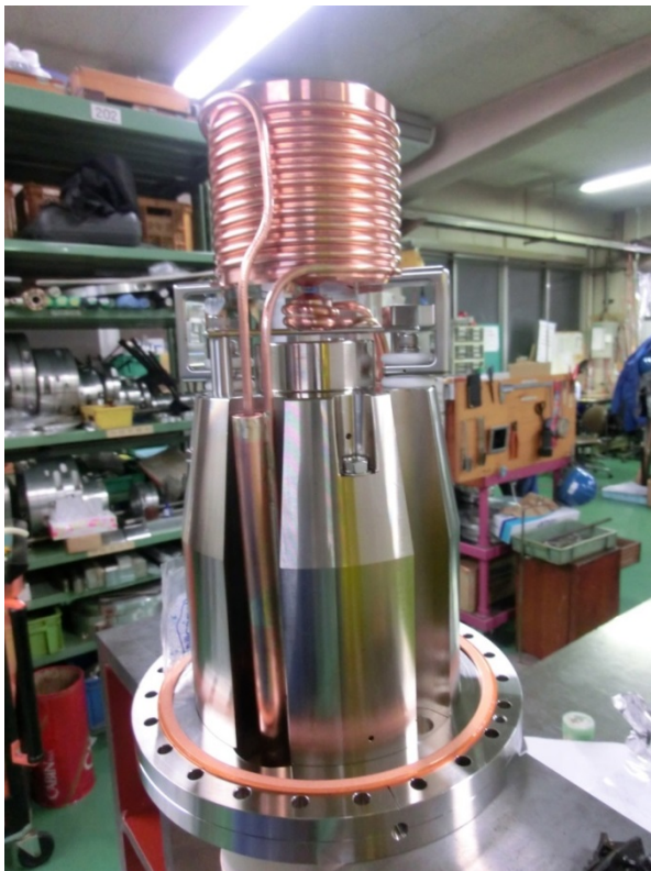
Figure 4: New positron source. At the top is the flux concentrator. Below the concentrator, a positron target can be seen.
