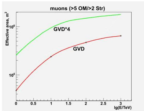
Figure 2: Muon effective area. The curves labeled by GVD\*4 and GVD correspond to configurations with 10368 OMs and 2304 OMs, respectively.
