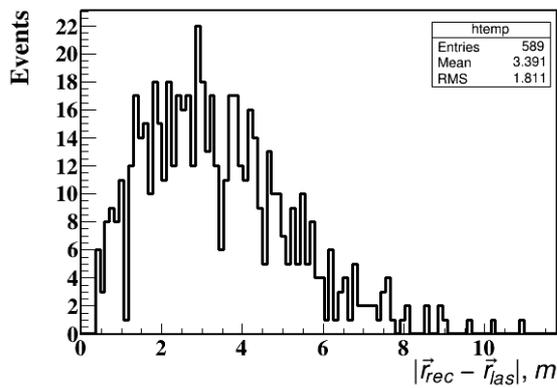
Figure 9: Deviation of reconstructed laser coordinates from those obtained by the acoustic positioning system.
