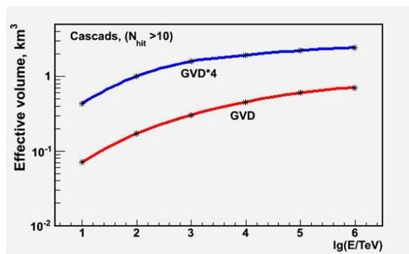
Figure 3: Effective volume of cascade detection. The curves labeled by GVD\*4 and GVD correspond to configurations with 10368 OMs and 2304 OMs, respectively.
