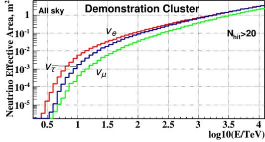
Figure 4: Neutrino effective areas for each flavor averaged over all arrival angles. The effective area includes effects from attenuation of neutrinos in Earth.
