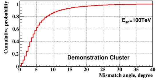
Figure 5: The fraction of shower events with mismatch angle less than a given value.
