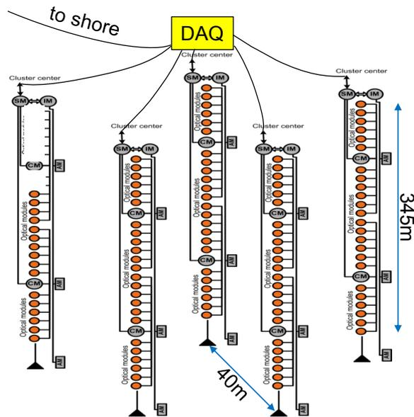
Figure 7: Schematic drawing of the second stage of the demonstration cluster.
