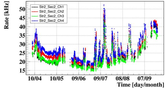
Figure 8: Counting rates of four OMs on the top section of the second string which were observed in 2014.
