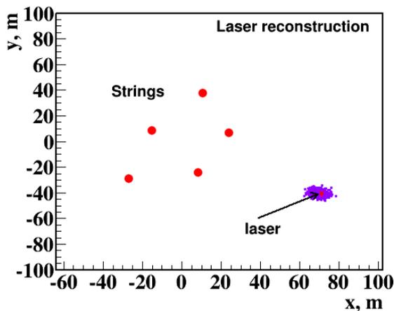
Figure 10: Top view of reconstructed laser positions. The star indicates the laser position obtained by the acoustic system.
