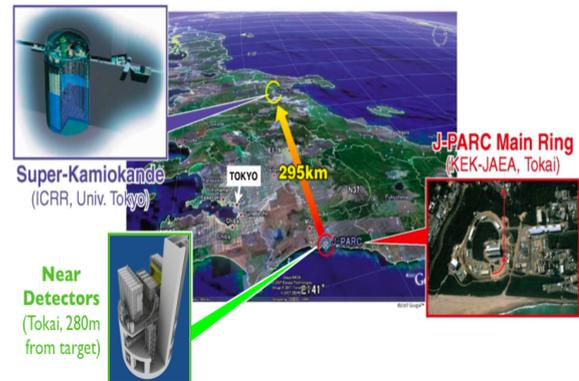
Figure 1: Layout of the T2K experiment, showing the position of the J-PARC accelerator complex where the muon neutrino is produced, the near detectors located at 280 m from the production target and the far detector Super-Kamiokande, situated 295 km away.
