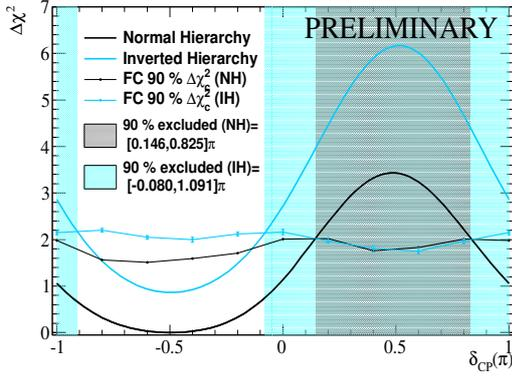
Figure 4: Profiled  $\Delta\chi^2$  as a function of  $\delta_{CP}$ , result of the T2K joint 3-flavour Frequentist analysis combined with the results of the reactor experiments. The critical  $\Delta\chi^2$  values and excluded regions obtained at the 90% CL for the normal and inverted hierarchies are overlaid.
