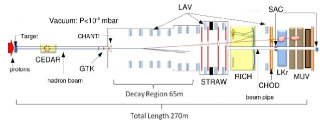
Figure 2: Layout of the NA62 experiment at CERN.
