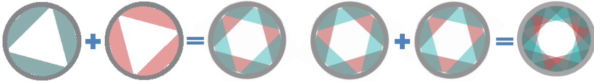
Figure 3. Assembly of a tracker station. Six panels of 96 groups of straws are assembled into a panel. Two panels form a tracker station.
