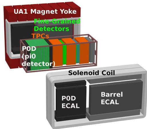
Figure 2: Schematics of ND280 in the opened magnet position. The tracker is visible next to the POD, with its 3 TPCs and 2 FGDs represented in fake color for display purposes.
