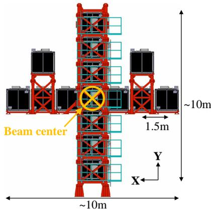
Figure 1: Schematics of the INGRID apparatus. The central cross is composed of 7 standard modules in the horizontal segment, and 7 in the vertical one.
