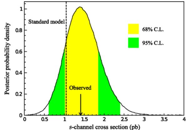
Figure 8: Lepton plus jets analysis: posterior probability density distribution for the  $s$ -channel cross section measurement, with the SM prediction shown as the vertical dashed line.
