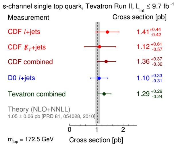
Figure 10: Summary of the Tevatron single top  $s$ -channel cross section measurements. The grey vertical line is the theoretical cross section value with uncertainties.
