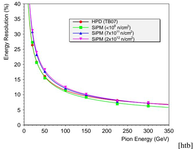
Figure 2: Energy resolution as a function of pion energy for neutron-irradiated SiPMs (from simulations) compared to HPDs (from test beam data). A 1 mm<sup>2</sup> device is shown [6].
