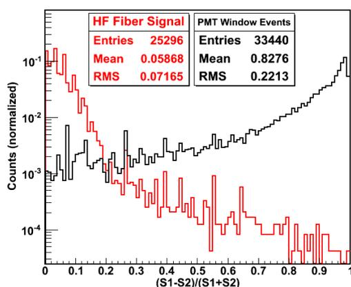
Figure 4: Identification variable for anomalous signals using two anode readout. S1 and S2 represent the signals in the two readout channels, with  $S1 > S2$ . Data collected from CERN H2 test beam. Black distribution is from particle hits on the PMT, while the red curve is from electron showers [6].
