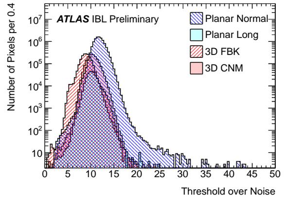
Figure 5: Threshold over noise distribution of pixels for 1500 e<sup>-</sup> threshold tunings at -12°C module temperatures for 18 staves. The bump around a threshold to noise value of 5 is caused by a noise on HV lines of the setup and the sensitivity of FBK modules to such noise. The fraction of noisy IBL pixels is less than 0.03% [7].
