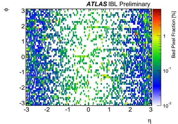
Figure 8: The bad pixel fraction in the  $\eta - \phi$  plane for the 14 IBL staves. It represents the inefficiency map of the IBL as it is installed [7].
