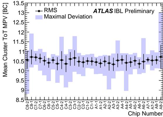
Figure 7: The average most probable cluster ToT value obtained from a Landau-Gauss fit as a function of the chip number for source scans performed at 22°C with a 3000  $e^-$  threshold and 10 BCs ToT at 16000  $e^-$  tuning [7].
