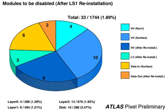
Figure 2: Number of modules of the Pixel Detector to be disabled after re-installation in the ATLAS Experiment classified by the failure mode (HV/LV/Data In/Data Out) and the phase of causing problems (Run1/ Surface / After re-installation). Modules having issues but being operable are not included [4].
