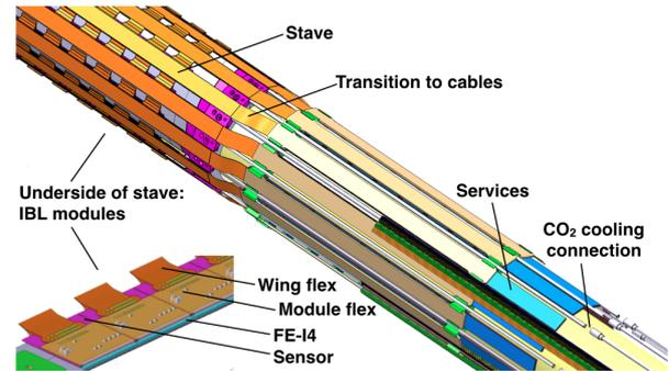
Figure 3: A longitudinal view of IBL mounted on the beam-pipe with connections to services and a sketch of an IBL stave with IBL modules loaded.
