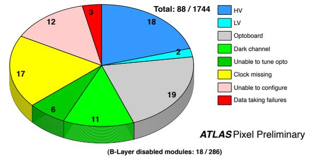
Figure 1: Number of disabled modules of the Pixel Detector at the end of Run1 classified by the type of failure [4].
