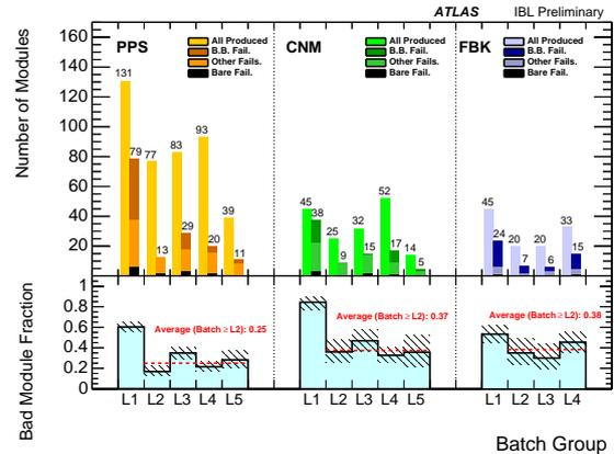
Figure 4: Yield of IBL module production for sensor types of Planar (PPS) and 3D (CNM, FBK) per production batch group. In the top panel for failure modules, B.B. Fail. stands for the large bump-bonding failure, Bare Fail. stands for the module not assembled due to mainly mechanical damages, and Other Fails. stands for both electrical and sensor failures discovered after the assembly [4].
