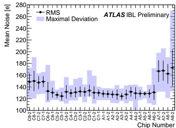
Figure 6: Average threshold noise distribution among the 18 production staves after tuning all pixels to a target threshold of 1500 e<sup>-</sup> and to a 10 ToT target response for 16000 e<sup>-</sup> at -12°C module temperature. The error bars show the RMS spread, while the solid boxes show the minimum and maximum values [7].
