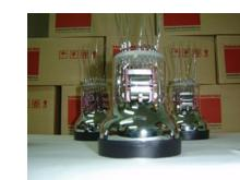
30 units from Hamamatsu R12669 PMT (specially built for ANAIS) have been received at LSC by now (the remaining 10 before Aug 2014) and are being characterized (radiopurity, dark current, gain, quantum efficiency...)
