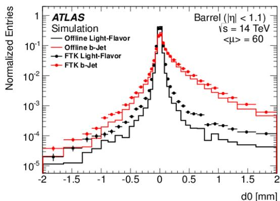
Figure 7: The transverse impact parameter for tracks associated to light-flavor (black) and heavy-flavor (red) jets. The solid lines show the distribution for the offline tracks, whereas the points show the FTK tracks [13].
