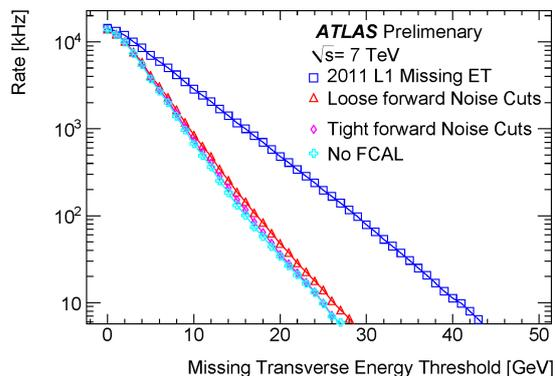
Figure 3: Level-1 MET rates as a function of threshold, for several pile-up noise cut scenarios. The 2011 configuration corresponds to noise cuts of  $\sim 1\text{ GeV}$ . The loose forward noise cut applies cuts in the first Forward Calorimeter (FCAL) layer and in the second layer at  $|\eta| > 3.5$ . The tighter noise cuts raise these by maximum 1 GeV, and the final case removes FCAL entirely from calculation. At Run-1 luminosity, the bulk reduction is achieved with the loose cuts [7].
