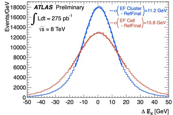
Figure 6: The resolution of the MET  $x$  component for 2012 data for EF, calculated as residuals with the offline measurement, for two different algorithms: in blue the EF topological cluster calculation and in red the EF cell based calculation [11].
