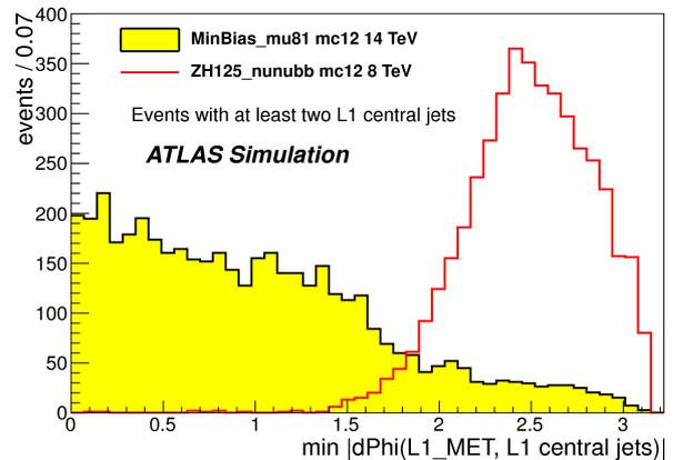
Figure 5: Minimum azimuthal angular distance between L1 MET and central jets with  $p_T > 20$  GeV and  $|\eta| < 2.5$  for minimum bias and ZH events with at least two central jets [8].
