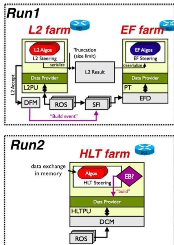
Figure 2: Schematic view of the structure of the HLT code, as used for Run-1 (top) and for Run-2 (bottom). The simplified network architecture, with one HLT farm, is reflected into a merged L2/EF infrastructure, more simple and compact. The Steering is the module scheduling the algorithms, while the Data Provider accesses the data from the ROSes.
