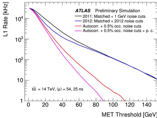
Figure 4: The estimated L1 MET trigger rate as a function of threshold, from 14 TeV minimum bias Monte Carlo. Shown are the operation scenarios with 2011 and 2012 noise cuts using matched FIR filters and two options for Run-2 with noise cuts optimized for 0.5% occupancy, using auto-correlation FIR filters with and without pedestal correction (p.c.) which are possible with the upgraded L1 calorimeter trigger system [9].
