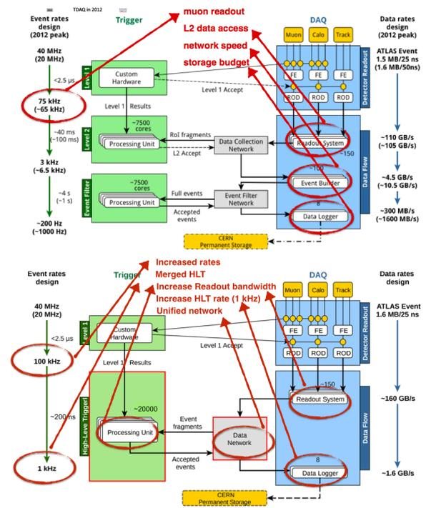
Figure 1: Overview of the ATLAS TDAQ architecture during Run-1 (top) and Run-2 (bottom), showing both the design values of latencies and sustained rates and the maximum reached during Run-1. The bottlenecks and the expected values for Run-2 are also pointed out.
