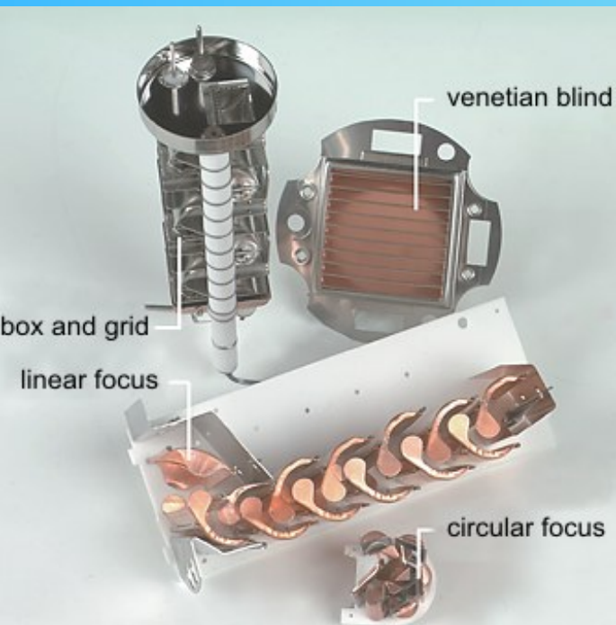
Fig. 4-8. Configurations of some common types of PM tubes. (a) Focused linear structure. (b) Circular grid. (c) Venetian blind. (d) Box-and-grid. (Courtesy of EMI GENCOM Inc., Plainview, NY.)
