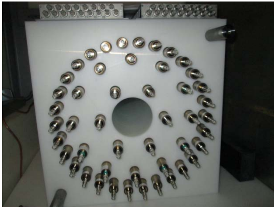
Counters embedded in a polyethylene matrix
