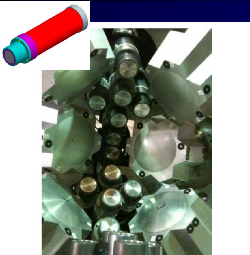
Figure 2: Configuration of \text{LaBr}_3:\text{Ce} detectors within EURICA.
