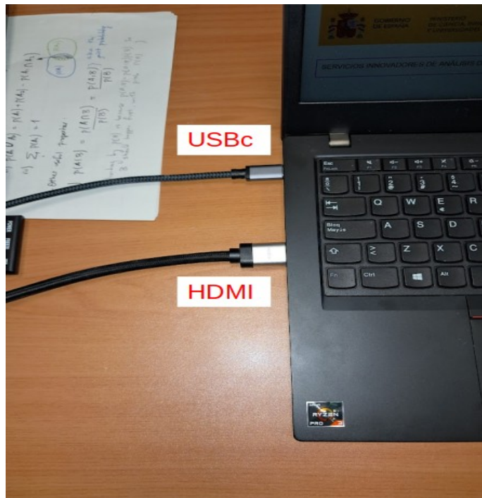
Figure 2: The laptop is connected to a central hub that controls speakers/microphones/cam/ethernet
